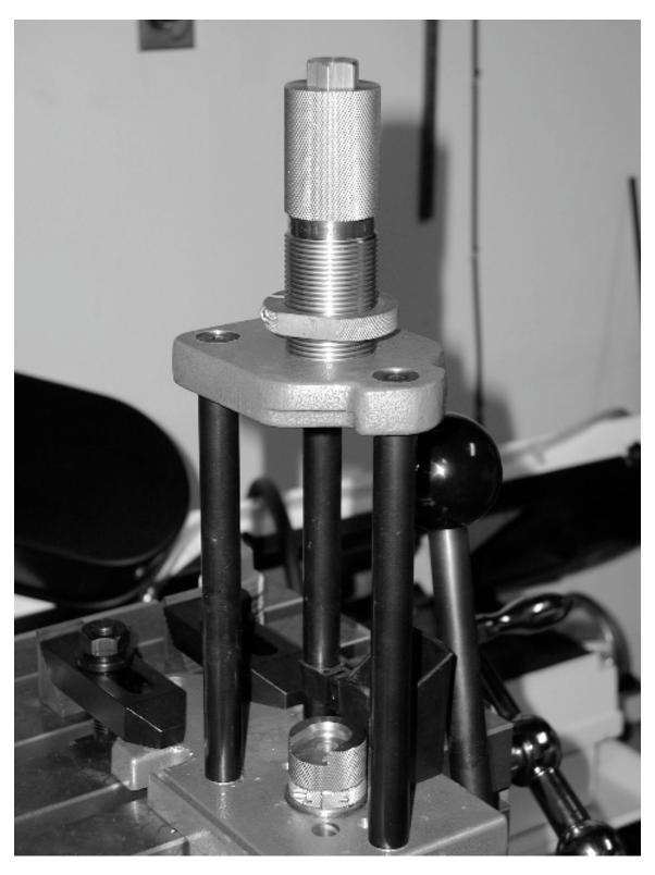
3. Thread the .50 BMG Match FL Sizer into the press part way.
