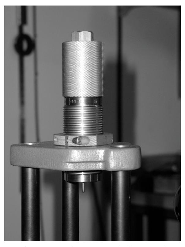
6. Lower the press ram, screw the primer seater in 1/8 additional turn and secure the lock ring.
