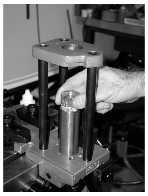
1. Put a .50 BMG shell holder in the press and lock it down.
