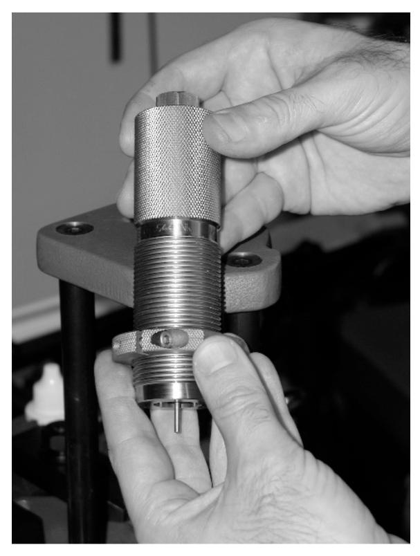
2. Install a lock ring on the .50 BMG Match FL Sizer, but don't lock it down yet.
