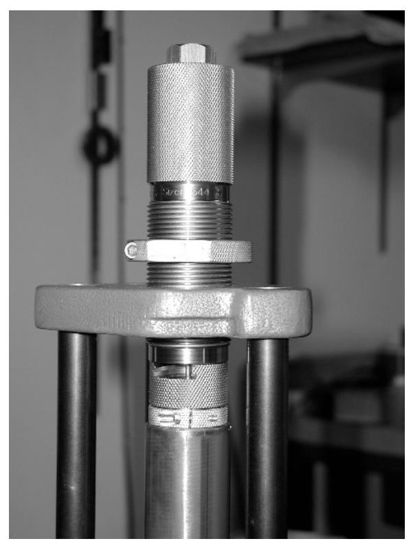
5. Screw the .50 BMG Match FL Sizer into the press until it just contacts the shell holder.
