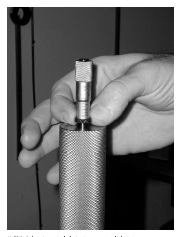
11. Unlock the micrometer lock ring (turn counter clockwise).
