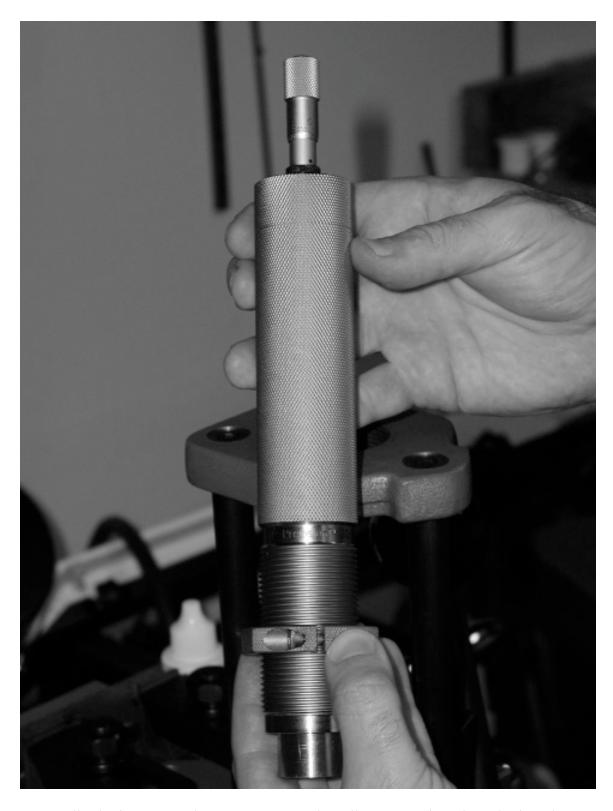
6. Install a lock ring on the .50 BMG Match Bullet Seater, but don't lock it down yet.
