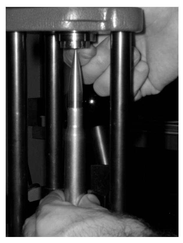
17. Remove the loaded round. Don't forget that you may need to lift up on the chamber sleeve to clear the bullet.
