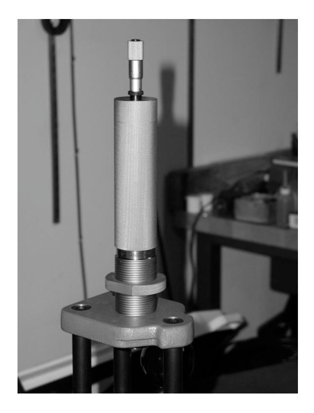
7. Thread the .50 BMG Match Bullet Seater into the press part way.
