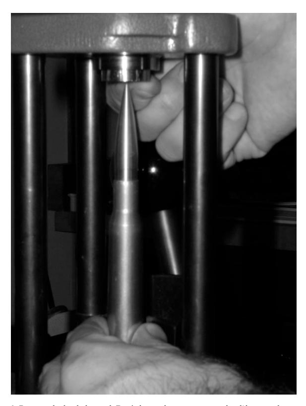
3. Remove the loaded round. Don't forget that you may need to lift up on the chamber sleeve to clear the bullet.
