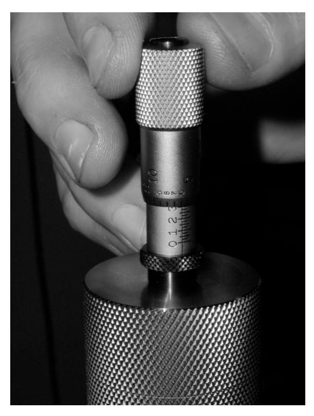
15. Turn the micrometer until resistance is felt.
