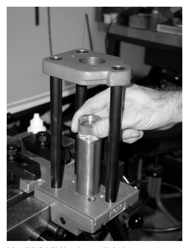
5. Put a .50 BMG shell holder in the press and lock it down.
