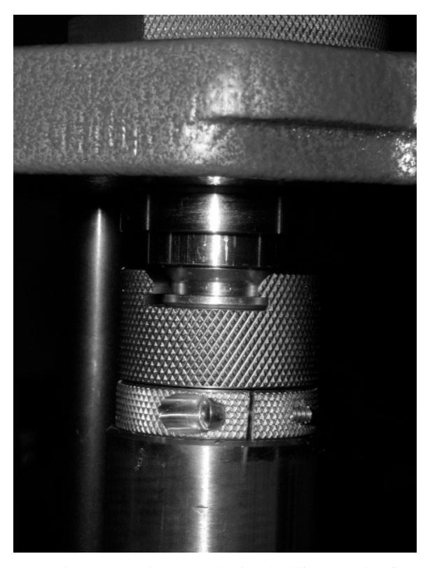
14. Raise the press ram to the top. Note that there should be a nominal .025'' gap between the shell holder and the chamber sleeve.
