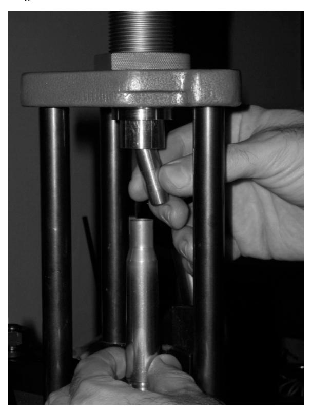
1. Place a primed and charged case in the shell holder. Set the bullet on top of the case.
