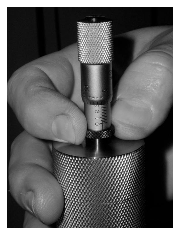
16. Lock the micrometer lock ring (turn clockwise). The micrometer setting, at this point, will be close to duplicating the OAL of the loaded sample round.
