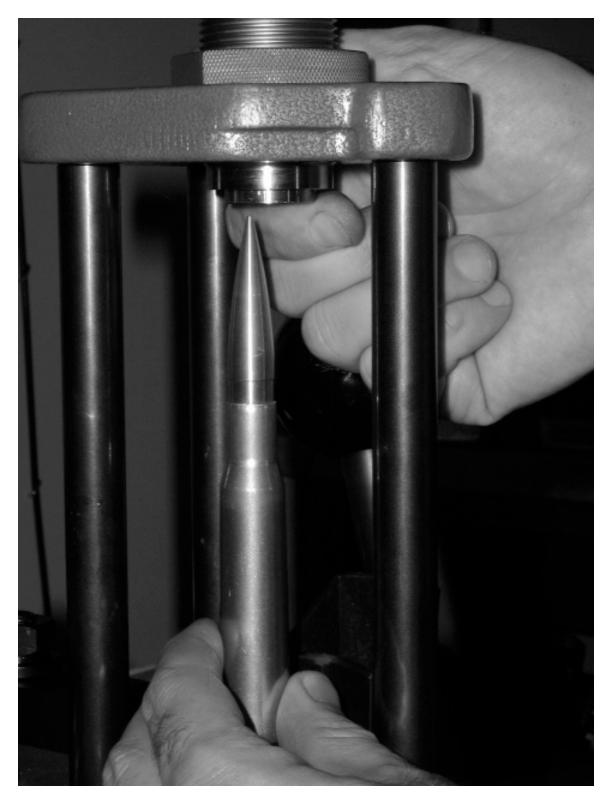
13. Put a loaded sample round in the press. You may need to lift up on the chamber sleeve to clear the bullet.
